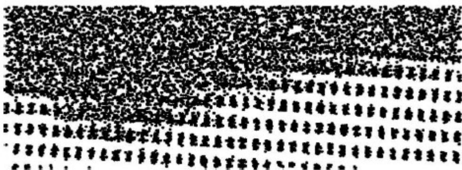
FIG. 4. Example of interface roughening occurring during crystal growth at the (13,12,11) interface for an undercooling of 40 K.
