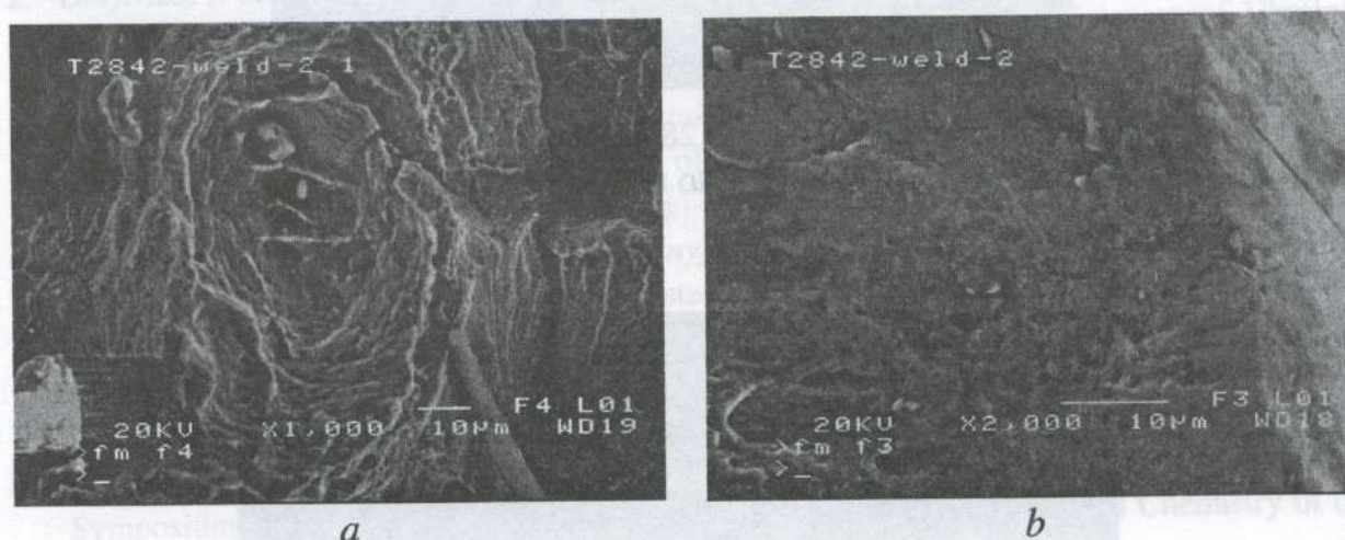
Fig. 3. Fracture character of the WJ specimen 2842 during the crack propagation perpendicular to WJ: a – \times 1000 ; b – \times 2000 .
