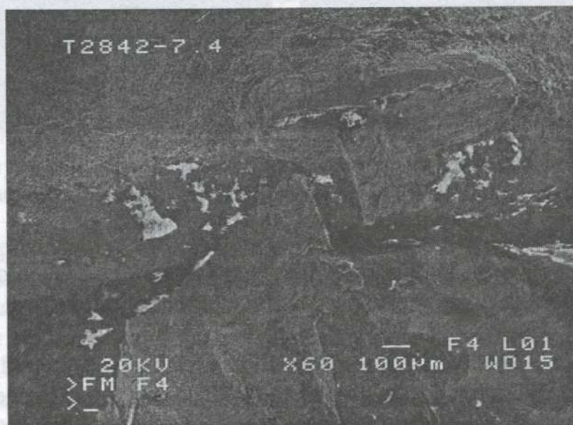
Fig. 5. Character of cracks branching during the passing of main crack Through the WJ-PM border in the 2842 specimen.
